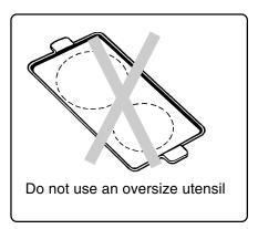
Specialty pans such as woks, lobster pots, pressure cookers, griddles, French fryers, etc. must meet similar design requirements as regular cookware: flat bottom, balanced, correct size, and proper cover (if applicable). Do not use utensils such as griddles, roasting pans, au gratin pans, fish poachers or other cooking utensils that must fit across two burners. Use of these products can result in damage to the glass cooktop and porcelain burner pans.
